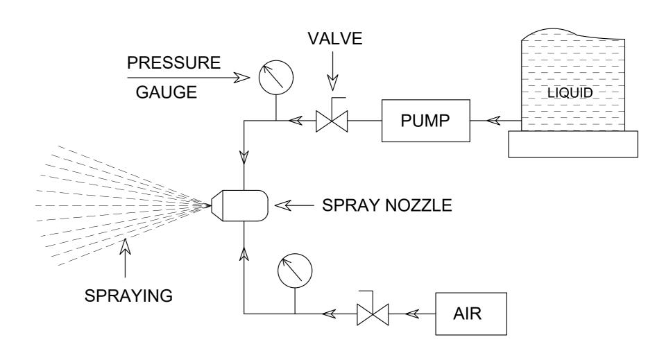
BASIC DESIGN AIR ATOMIZING NOZZLES
