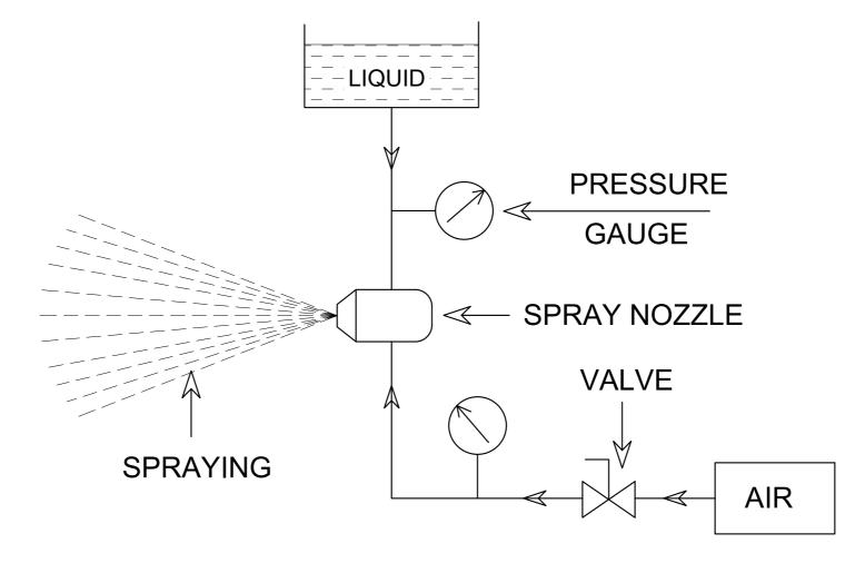
**3) Siphon Method**: In this method of liquid supply, The liquid is feed by the suction of liquid from a certain siphon height of liquid by pressurized Air ,This method is basically used where liquid tank and motor pump is not available for liquid feeding.
