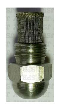
JSR Oil Spray Nozzles are design with Semi Hollowcone Spray pattern, It has a Swirl Insert part permitting flow only through the slot of the Insert . This Oil spray Nozzles are Assembled with Extra fine mesh filter in order to provide highly efficient in depth filtration .
