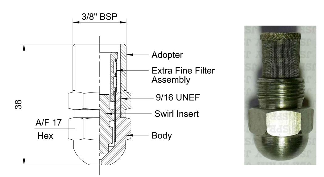
JSR Oil Spray Nozzles are design with Semi Hollowcone Spray pattern, It has a Swirl Insert part permitting flow only through the slot of the Insert . This Oil spray Nozzles are Assembled with Extra fine mesh filter in order to provide highly efficient in depth filtration .
